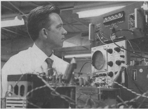
BREADBOARD MODEL of an untried circuit for a new production tester is constructed by Jim Gris-
